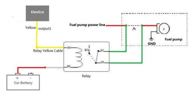
Note: To implement remote fuel and power cut-off, connect the relay to the fuel pump cable or the engine cable in series.
