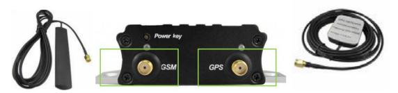
Connect the GSM antenna to the SMA connector which is 'GSM' text labelled. The GSM antenna is non-directional, so you can hide it in any place of vehicle.
